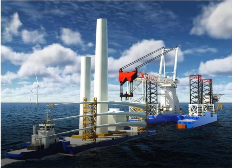
With a crane capacity of 3,000 tons and a crane hook height of up to 182 meters above deck, FEEDERDOCK is designed to install the 25 MW wind turbine generation including foundations up to 2,800 tons. Its leg length of 131 meters grants the ability to cope with water depths of up to 70 meters.
